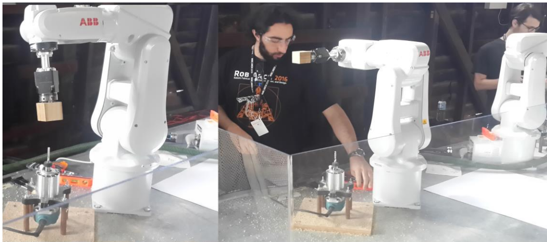
Fig.09 The Robotic Joints Fabrication: (Right) the starting point of the robot after manual fixation of joint on its tip, (left) the robot while fabrication after reading the joint data Reference: Photographed by the author March 2016 at Dynamo-Build Workshop, Sydney
